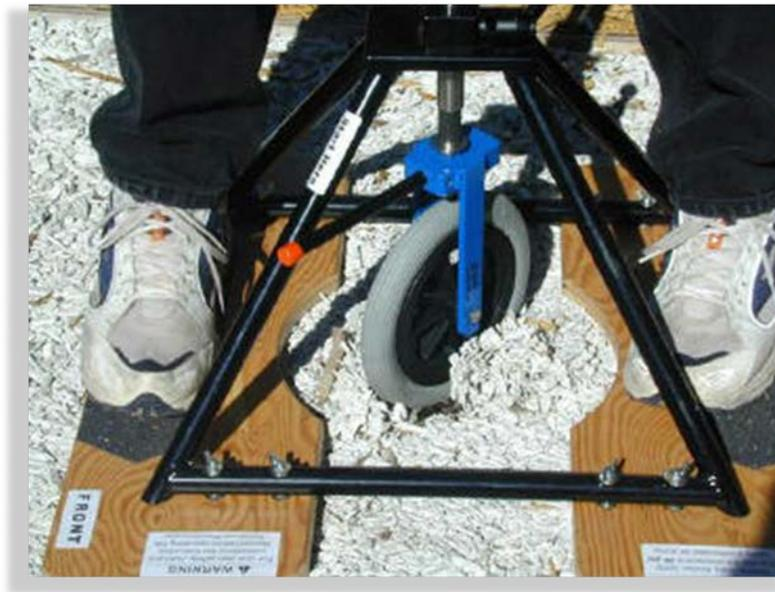
Rotational Penetrometer twisting to measure stability
